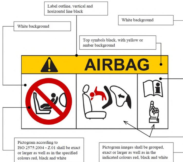
The overall dimensions of the label shall be at least 120 x 60 mm or the equivalent area : see 1<sup>st</sup> stage approval
